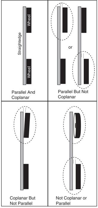
Figure 22. Wheel alignment and misalignment examples.
